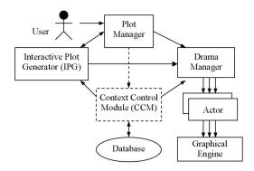
Figure 2: LOGTELL's architecture (arrows represent dataflow)
