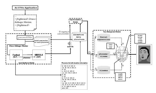
Figure 3: An overview of the ETH architecture and its submodules.
